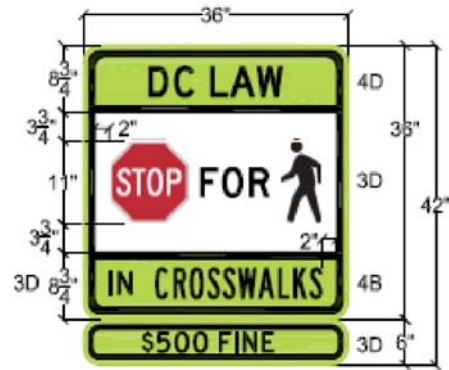
Side of Street Pedestrian Crossing Sign R1-6a(1)
